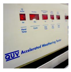
o The QUV is a 48 standard size specimen holder that is capable of producing the damage caused by sunlight, rain and due. Within a few days or weeks, we can reproduce the damage that occurs over months or years in South Africa.
